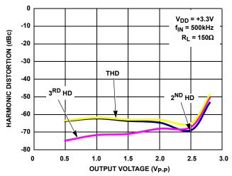
FIGURE 16. HARMONIC DISTORTION vs OUTPUT VOLTAGE
