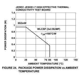
**Typical Performance Curves**  $V_{DD}$  = +3.3V,  $R_L$  = 150 $\Omega$ , unless otherwise noted (Continued)
