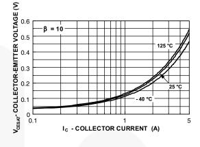
Figure 2. Collector-Emitter Saturation Voltage vs.
