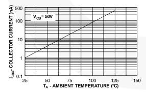
Figure 5. Collector Cut-Off Current vs.
