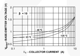
Figure 3. Base-Emitter Saturation Voltage vs.
