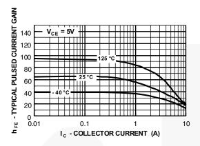
Figure 1. Typical Pulsed Current Gain vs.
