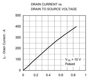
V<sub>DS</sub> - Drain to Source Voltage - V
