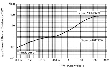
TRANSIENT THERMAL RESISTANCE vs. PULSE WIDTH
