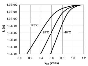
Figure 6: Body-Diode Characteristics (Note E)
