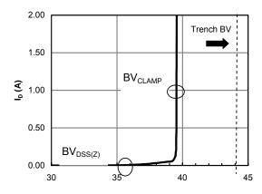
$\label{eq:VDS} V_{DS} \, \mbox{(Volts)}$  Fig 15:  $BV_{CLAMP} \, \mbox{Characteristic}$
