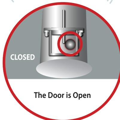
Because the magnet ball contact will not weld, when the door is opened the contact will close and the **SYSTEM WILL ALARM**.
