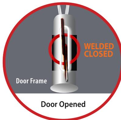
Reed contacts operate by magnetic induction, so they are not attracted to the door magnet.
