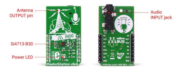
The click is designed for communication over the I2C/2-wire control interface. When selecting 2-wire mode, SCLK pin should stay at a HIGH logic level during the rising edge on the RST pin, and stay HIGH until after the first start condition. Also, a start condition must not occur within 300nS before the rising edge on the RST pin. The 2-wire bus mode uses only the SCL and SDA pins for communication.
