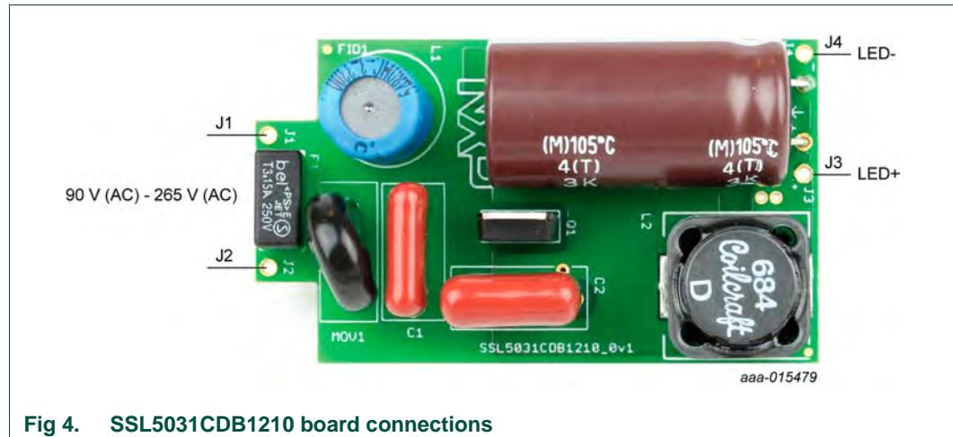
Fig 4. SSL5031CDB1210 board connections
