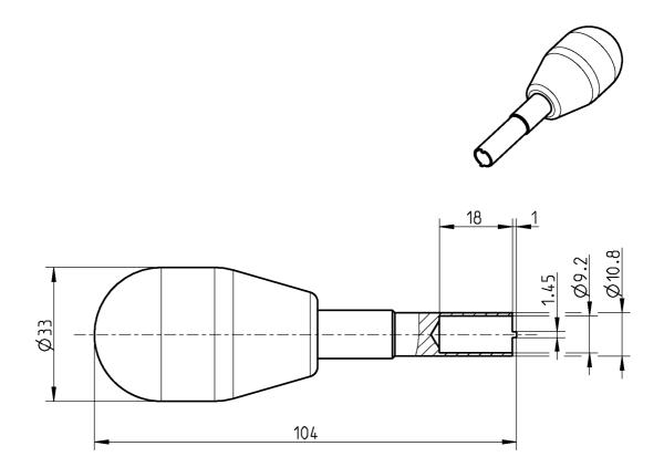
All dimensions are in mm; tolerances according to ISO 2768 m-H
