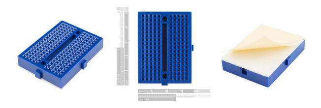
**Description:** This blue Mini Breadboard is a great way to prototype your small projects! With 170 tie points there's just enough room to build and test simple circuits; They're also great for breaking out DIP package ICs to jumper wires! If you run out of room, no worries, these mini breadboards can be snapped together to form larger stretches of board. It has a peel and stick adhesive backing as well as two mounting holes for M2 screws so you can anchor it down.
