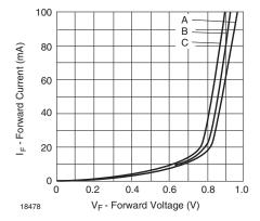
Fig. 2 - Typical Forward Conduction Curve
