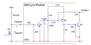
Figure 40. Circuit configuration for using negative On/Off
