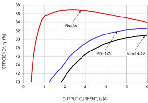
Figure 7. Converter Efficiency versus Output Current.
