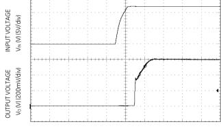
Figure 5. Typical Start-up Using On/Off Voltage ( $I_0 = I_{o,max}$ ).
