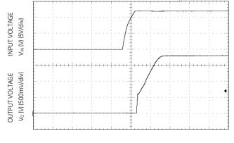
Figure 17. Typical Start-up Using On/Off Voltage ( $I_0 = I_{0,max}$ ).
