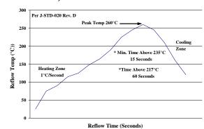
Figure 51. Recommended linear reflow profile using Sn/Ag/Cu solder.
