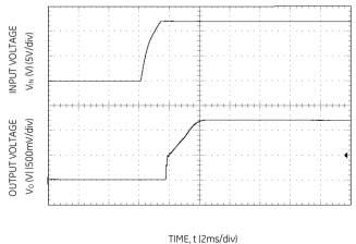
Figure 12. Typical Start-up Using Input Voltage ( $V_{IN} = 12V$ ,  $I_0 = 1...$
