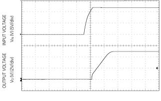
Figure 35. Typical Start-up Using On/Off Voltage ( $I_0 = I_{o,max}$ ).
