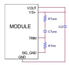
Figure. 47. Circuit diagram showing connection of  $R_{\text{TUME}}$  and  $C_{\text{TUNE}}$  to tune the control loop of the module.
