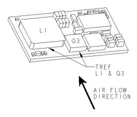
Figure 50. Preferred airflow direction and location of hotspot of the module (Tref).
