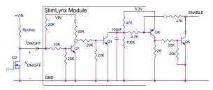
Figure 39. Circuit configuration for using positive On/Off logic.
