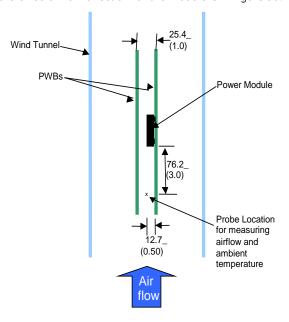
Figure 49. Thermal Test Setup.
