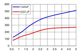
Figure 37. Input ripple voltage for various output voltages with 1x22 µF or 2x22 µF ceramic capacitors at the input (6A load). Input voltage is 12V.
