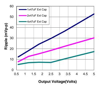
Figure 38. Output ripple voltage for various output voltages with external 2x47  $\mu$ F, 4x47  $\mu$ F, 6x47  $\mu$ F or 8x47  $\mu$ F ceramic capacitors at the output (6A load). Input voltage is 12V.
