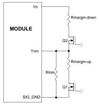
Figure 43. Circuit Configuration for margining Output voltage.
