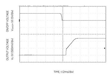
Figure 11. Typical Start-up Using On/Off Voltage ( $I_0 = I_{o,max}$ ).
