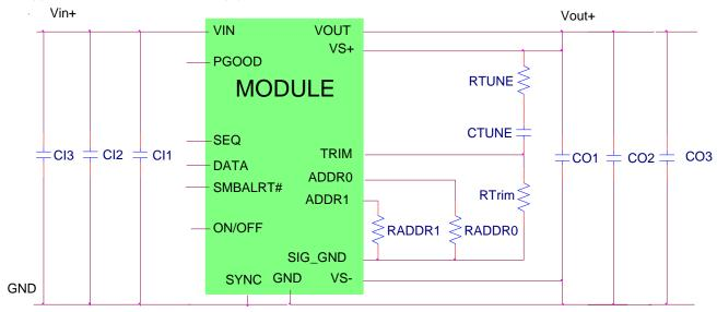
CI1 Decoupling cap - 1x0.047µF/16V ceramic capacitor (e.g. Murata LLL185R71C473MA01)
