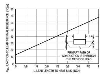
Figure 10. Typical Thermal Resistance
