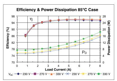
**Figure 8** – Efficiency and power dissipation at  $T_C = 85^{\circ}C$
