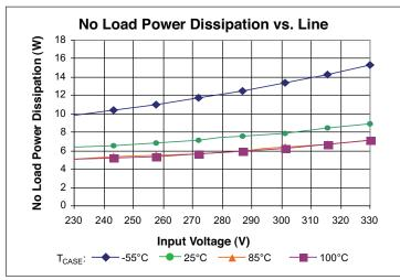
Figure 2 – No load power dissipation vs.  $V_{IN}$
