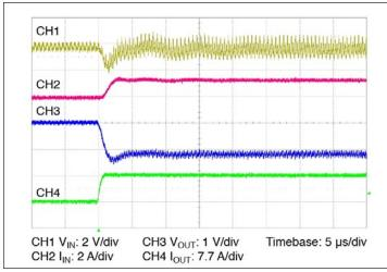
**Figure 13** – 0 A– 6.25 A transient response:  $C_{IN} = 100 \ \mu$ F, no external  $C_{OUT}$
