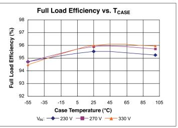
Figure 3 – Full load efficiency vs. full T<sub>MAX</sub> range
