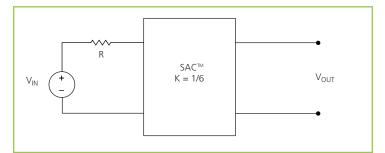
**Figure 15** – K = 1/6 Sine Amplitude Converter<sup>TM</sup> with series input resistor
