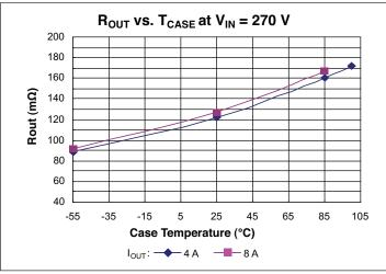
Figure 9 – R<sub>OUT</sub> vs. temperature
