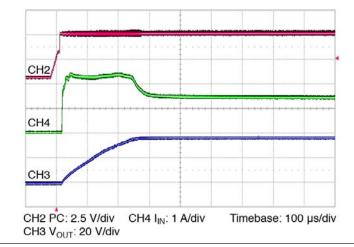
**Figure 12** – Start up from application of PC;  $V_{IN}$  pre-applied  $C_{OUT} = 50 \ \mu F$
