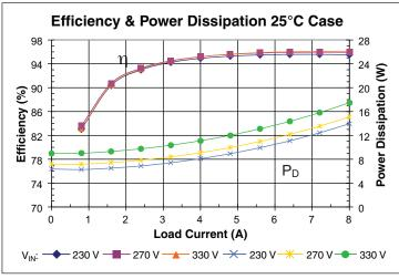
**Figure 6** – Efficiency and power dissipation at  $T_C = 25^{\circ}C$
