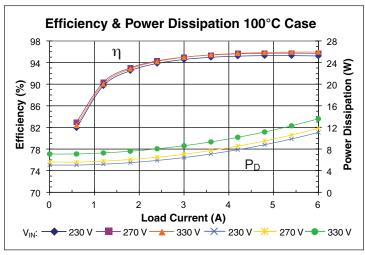
**Figure 7** – Efficiency and power dissipation at  $T_C = 100^{\circ}C$
