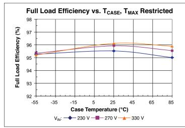
Figure 4 – Full load efficiency vs. T<sub>MAX</sub> restricted
