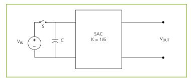
Figure 16 – Sine Amplitude Converter<sup>™</sup> with input capacitor
