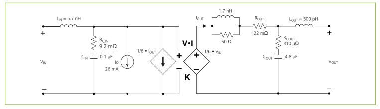
Figure 14 – V•I Chip<sup>™</sup> AC model
