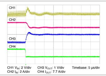
**Figure 14** – 6.25 A – 0 A transient response:  $C_{IN} = 100 \ \mu F$ , no external  $C_{OUT}$
