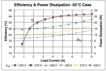
**Figure 5** – Efficiency and power dissipation at  $T_C = -55^{\circ}C$
