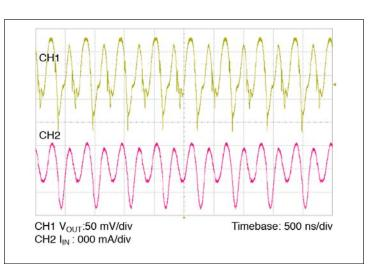
**Figure 11 –** Full load ripple, 100 μF C<sub>IN</sub>: No external C<sub>OUT.</sub> Board mounted module, scope setting : 20 MHz analog BW
