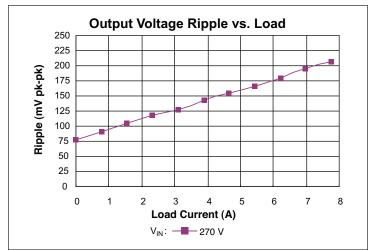
**Figure 10 –** V<sub>RIPPLE</sub> vs. I<sub>OUT</sub> ; No external C<sub>OUT.</sub> Board mounted module, scope setting : 20 MHz analog BW
