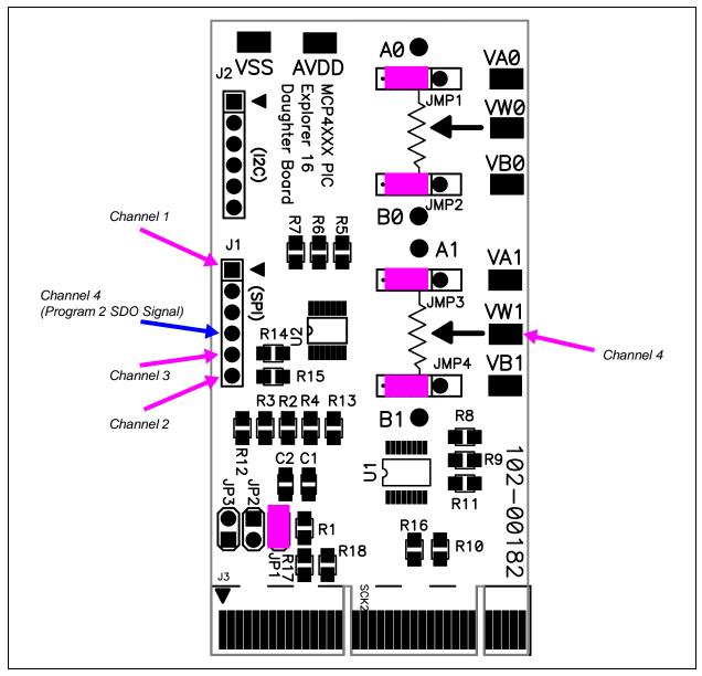
FIGURE C-1: Tested Jumper Configuration and Test Points.
