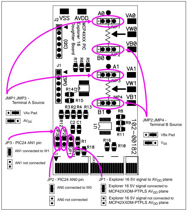
FIGURE 2-2: MCP42XXDM-PTPLS Jumper Configuration and Oscilloscope Test Points.
