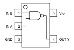
Figure 1. Pinout (Top View)
