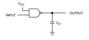
\*Includes all probe and jig capacitance. A 1–MHz square input wave is recommended for propagation delay tests.
