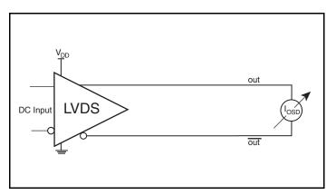
**Differential Output Short Circuit Setup**
