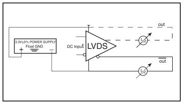
High Impedance Leakage Current Setup
