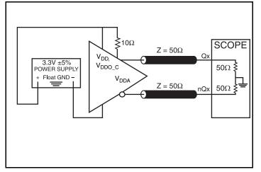
3.3V LVDS Output Load AC Test Circuit
