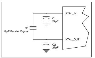
Figure 2. Crystal Input Interface
