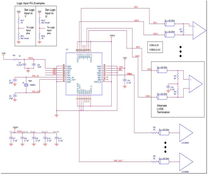
Figure 6.8402015 Schematic Example
