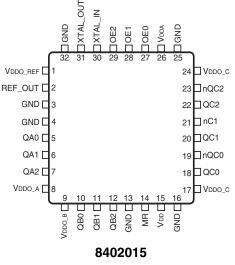
32-Lead VFQFN 5mm x 5mm x 0.925mm package body K Package Top View
