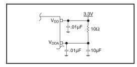
Figure 1. Power Supply Filtering
