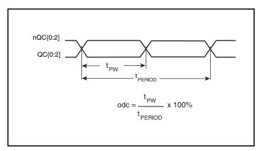
Differential Output Duty Cycle/Pulse Width/Period
