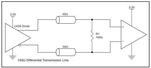
Figure 4. Typical LVDS Driver Termination
