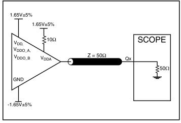
3.3V LVCMOS Output Load AC Test Circuit
