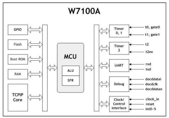
Figure 1.1 W7100A Block Diagram
