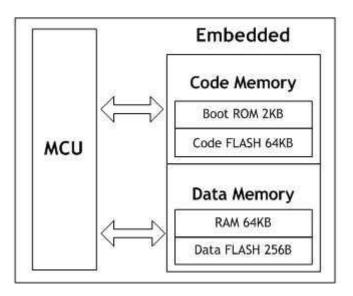
Figure 2.1 Code / Data Memory Connections
