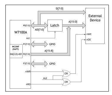
Figure 2.6 Standard 8051 External Pin Access Mode (EM[2:0] = "001")
