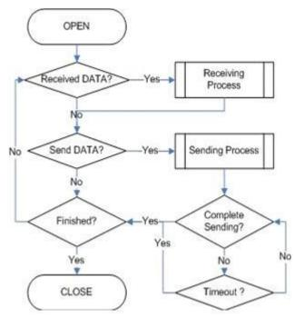
Figure 9.7 IPRAW Operation Flow
