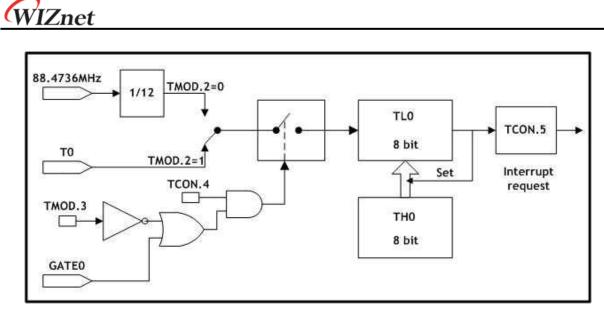
Figure 5.8 Timer/Counter0, Mode2: 8-Bit Timer/Counter with Auto-Reload
