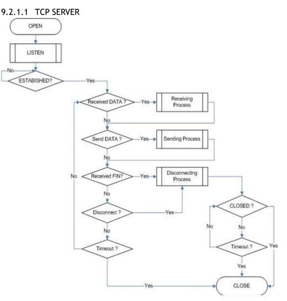
Figure 9.3 "TCP SERVER" Operation Flow
