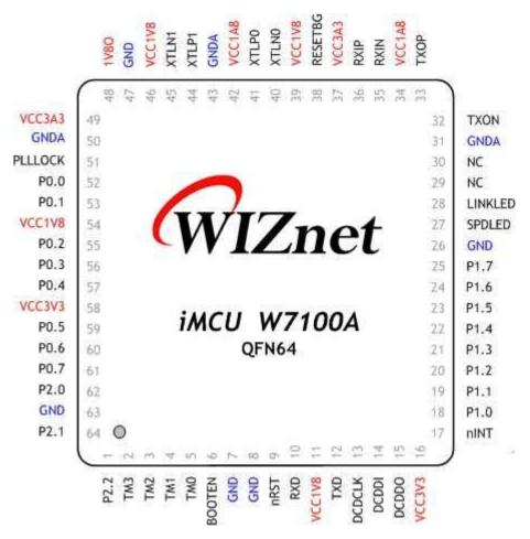
Figure 1.8 W7100A QFN 64 Pin Layout
