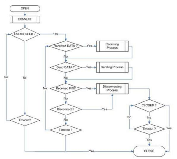
Figure 9.4 "TCP CLIENT" Operation Flow
