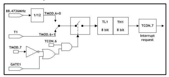
Figure 5.11 Timer/Counter1, Mode1: 16-Bit Timers/Counters
