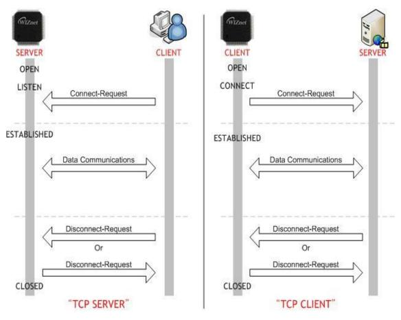
Figure 9.2 TCP SERVER & TCP CLIENT
