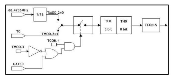
Figure 5.6 Timer Counter0, Mode0: 13-Bit Timer/Counter
