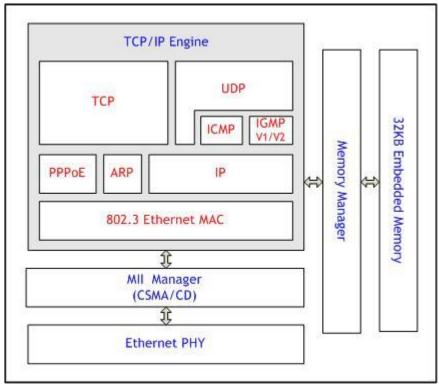
Figure 1.6 TCPIPCore Block Diagram
