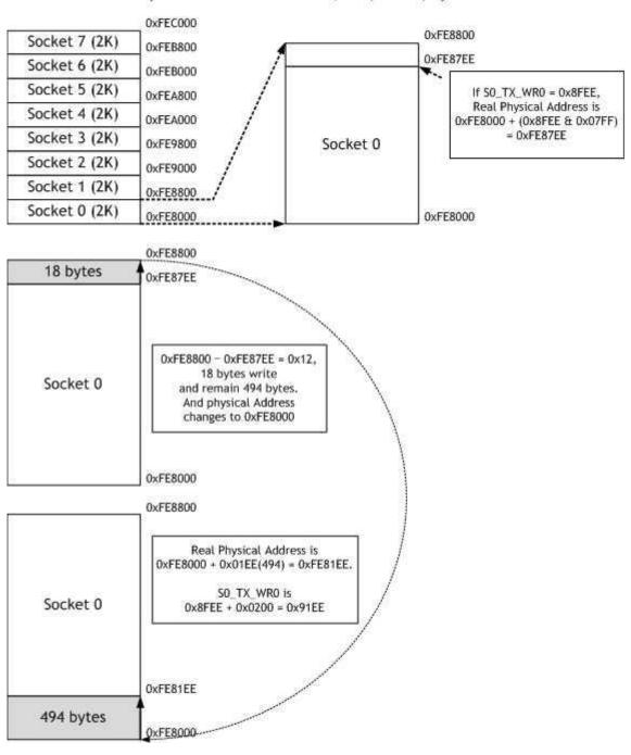
Chip Base Address = 0xFE0000, 512(0x0200) bytes send
