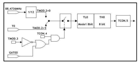
Figure 5.7 Timer/Counter0, Mode1: 16-Bit Timer/Counter
