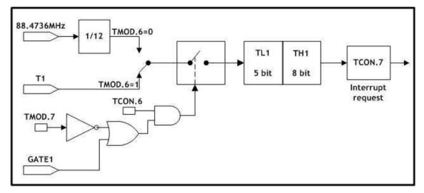
Figure 5.10 Timer/Counter1, Mode0: 13-Bit Timer/Counter
