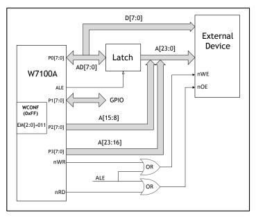
Figure 2.7 Standard 8051 External Pin Access Mode (EM[2:0] = "011")
