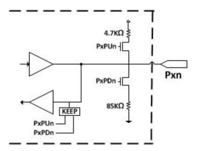
Figure 4.1 Port0 Pull-down register
