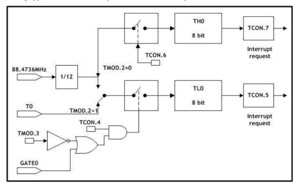
Figure 5.9 Timer/Counter0, Mode3: Two 8-Bit Timers/Counters
