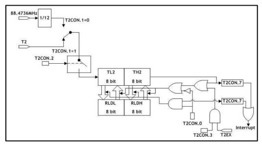
Figure 5.14 Timer/Counter2, 16-Bit Timer/Counter with Auto-Reload
