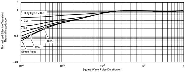
Normalized Thermal Transient Impedance, Junction-to-Case
