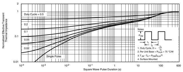
Normalized Thermal Transient Impedance, Junction-to-Ambient
