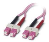
Assembled FO cable, zip cord cable, multi-mode fiberglass 50/125  $\mu$ m, OM4, plug: SC duplex/SC duplex, degree of protection: IP20, for installation in cable ducts or control cabinets, length: 2 m
